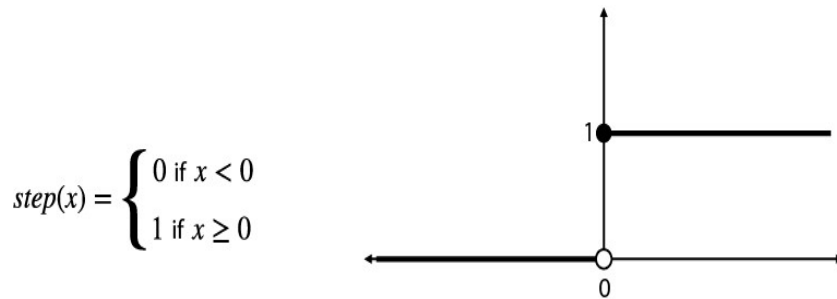
Figure B.4 The step function. For negative numbers it outputs 0, and for non-negative numbers it outputs 1.
